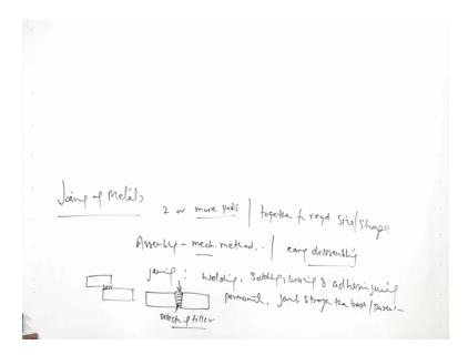
Now, we will come to the next topic that is about the joining of the metals. So, joining of the metals like the two or more parts are brought together for required for achieving the required size and shape.
