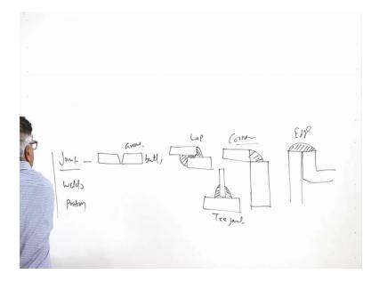
So, these are the basic aspects related with the joints, the there are different types of the joints which are used for the metallic continuity whatever is the kind of the joining process like brazing, shouldering or the welding or adhesive joining.
