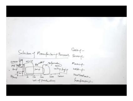
So, here if we see if you tried to put in this diagram in the x-axis we have volume starting with the say here it is a 0, 10, 100, 1,000, 10,000, 1,00,000 in the x-axis. And in the y-axis, we have the melting point temperature, so this is up to the 100, then up to say 1,000 then 10,000. So, for the metals, this is the range this is approximate range for the
