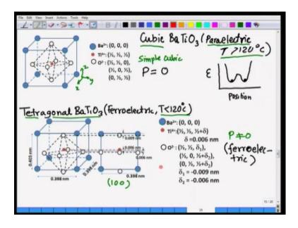
To understand ferroelectricity in barium titanate let us see it through this, this slide, this, these pictures I have put here and in order to understand ferroelectricity, let us start with this structure in barium titanate, which is not ferroelectric.
