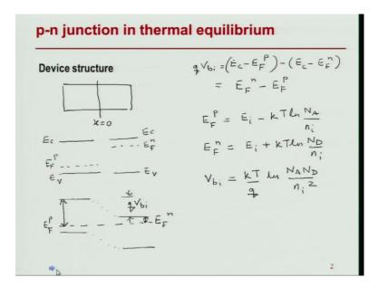
So, the next topic I am going to cover is the built-in potential in a p-n junction. How is the built-in potential in a p-n junction developed? So, already described by me, the device in the device structure, my device structure is defined in this manner. In one-dimension, at x is equal to 0 I have the junction and if I want to see, bring these two together, what would be the built-in potential?
