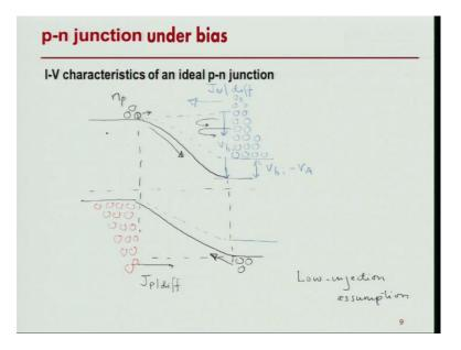
So, this is the bulk p-type region. In thermal equilibrium we had diffusion and drift current balancing each other in the depletion region. Now, if we forward bias it, effectively we are saying we have changed the built-in potential; we have reduced it, which was this earlier, by the applied bias. As a result, we can now see band bending is going to be different inside the depletion region due to this forward bias.
