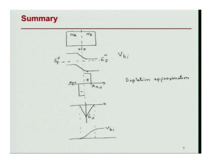
So, at this point I would like to summarize what we have learnt about the thermal equilibrium of the p-n junction. And so what we started with? We defined a p-n structure, which had uniform doping on both sides. Without getting into too much detail, we could calculate the built-in potential just from the requirement, that the, when I bring these two together, the fermi levels have to align on the n and the p side. From that we could calculate the built-in potential.
