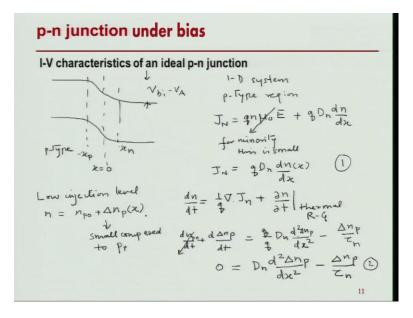
So, in the forward bias, where my built-in potential is reduced by the applied potential, I want to figure out what would be the current due to the forward bias. And as earlier, I am
