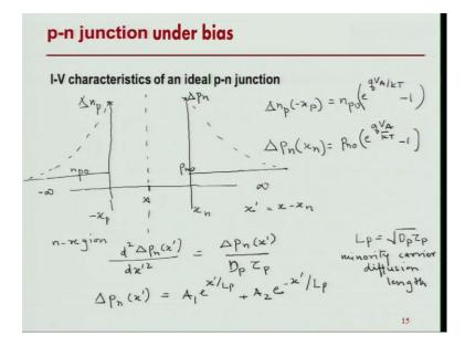
So, using this low, low level injection we have found the boundary conditions for my solution to the differential equations. This is the depletion region beginning and I have
