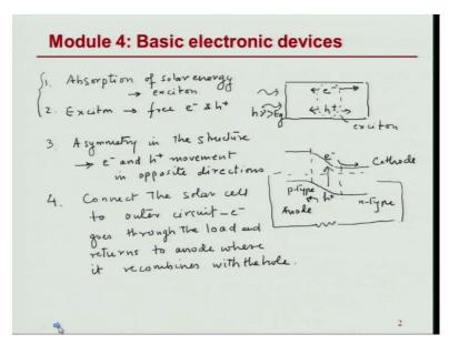
So, first we start with, what is a solar cell? So, as you can see the first step in solar cell is absorption of the solar energy and we have seen this earlier that if I have a semiconductor, by virtue of it is electronic structure, we can create a electron hole pair as long as the incoming energy that I am bringing is, is greater than the band gap of the semiconductor.
