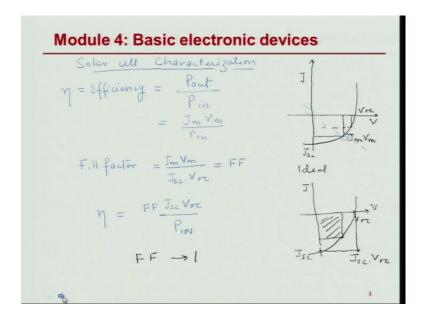
So, solar cell characterization is our next topic. Now, it is obvious solar cell is a energy conversion device. So, the main characterization for it must come from energy conversion and that is what it is, it is the efficiency of the solar cell and it comes from how much power I am collecting from my solar cell divided by how much power I am giving in the solar cell, that divides decides the efficiency of the solar cell.
