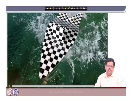
Now you see the ship is moving in a calm water and you can see that there are waves actually created by the ship because the ship is advancingly forwarding and then in the back side you can see there are some waves right this is typical problem wave resistance.
