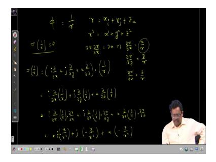
So, now first let us try to find out whether this  $\varphi$  1/r. I mean this  $\varphi$  ok this  $\varphi$  this function is 1 upon r whether this function is a velocity potential or not ok and the definition of r is nothing but xi +yj+ zk and therefore, this r square equal to nothing but x square plus y square plus z square right.
