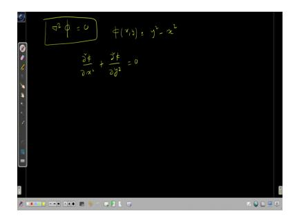
Now, before we proceed further try to find out a simple thing that the what is the meaning of a velocity potential? So, we can call the  $\varphi$  is a velocity potential if  $\nabla^2 \phi = 0$  right. This is how actually we say that whether this function is a velocity potential or not right.
