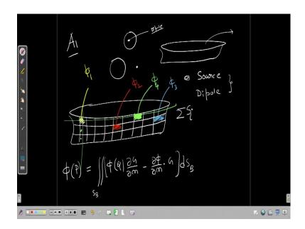
Now, if you remember that last class when I talked about that to find out the flow past cylinder and we put here a dipole right. And that means, that we claim that if we put a singular function instead of the body. So, you can have the same effect as if there is a body right, because we replace see we really do not put any cylinder when we talked about the flow past cylinder. We replace the cylinder and then place a dipole at in there right.
