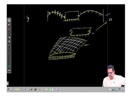
So, what happened? Finally, we have to either we need to model the free surface let us say and the boundary or we need to model only the body without the free surface. So, when I talked about this  $S_B$ . So basically, we are trying to say that we need to discretized either this whole thing or we need to discretize this one right.
