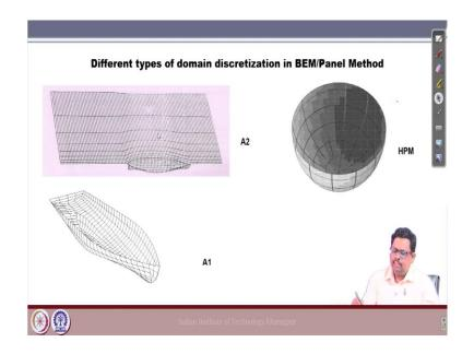
So, now, it is the same now we understand this all. Now, in case of  $A_2$ , we have to discretize the body as well as the free surface. In case of  $A_1$  we have to discretize the body only and in case of higher order panel, now we can see that these patches are really big comparison to the other two mesh right, ok.
