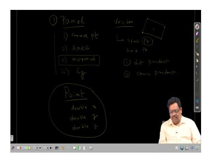
I could write some primitive class. So, first I can write one class which is called panel ok and then in this panel actually I can define some property of a panel. Now, how do I define a property of a panel? So, one panel is you know that it should be the coordinate of the 4 point. So, the property number 1, inside this I can put the you know the corner point. So, this is number 1.
