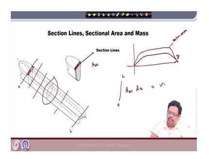
Now, you see here if I cut this, now here interestingly, if I cut in this plane, then definitely we are going to get some section line like this right. Now, here what are we going to do is from this section line, if I cut if you keep cutting, if I keep cutting over here, if I keep cutting over here, if I keep cutting over here; so, what you get? You get multiple section lines right.
