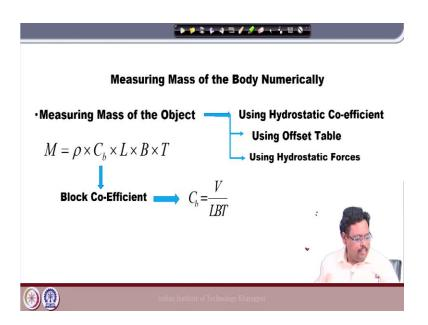
So, now, we are going to measure the mass of the body ok. So, how to get the mass of the body so, actually there are different way to measure it ok. So, first thing, we can use some hydrostatic coefficients or we can use some kind of offset table or we can use some hydrostatic forces with respect to the hydrostatic forces. So, we are going to discuss one by one all these three things ok.
