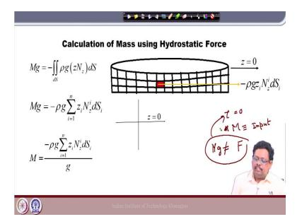
Then, what you going to do is let us take you take a patch, the mesh ok. So, once you take a patch or mesh, then you can calculate the hydrostatic force at that particular patch. Now, how you calculate the hydrostatic force? So, you can take the centroid of this patch right and then, you can define this as your  $z_i$ ; you can define this as your  $z_i$  right and then, you multiply it by  $\rho$  into g ok.
