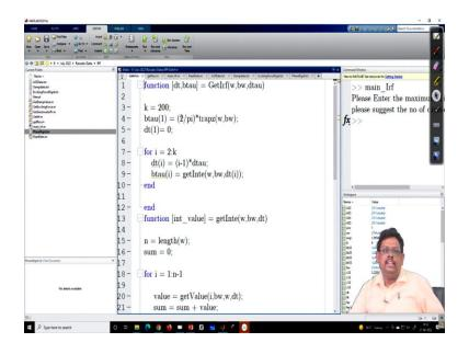
So, now if I look into this GetIrf this code, you can see at t equal to 0, I am using the trapezoidal rule. And then, here as I mentioned the previously when you write the code, this code should be written very neatly. I mean we do not need to write because if some unknown person will see your code, he should able to understand.
