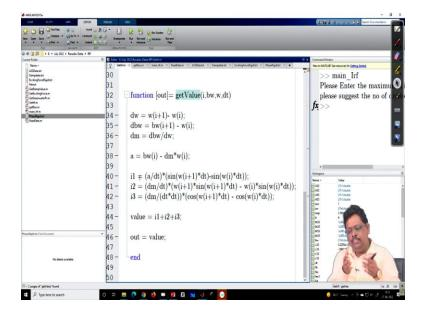
Now, here you can see this value I calculate here, right. So, you can see that  $d(\omega)$  I calculate, then this  $db(\omega)$  is nothing but the db and then this is the slope dm and this is the constant a. And then I have, you remember in my last class if you, last to last class I
