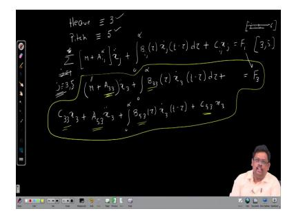
Now, here if you just because it is required to understand the code better way, here we have the coupled heave and pitch. So, we have heave and you can you make index the heave is 5, and then if you have the pitch, you can say the index of the pitch is 5. So, heave is 3 and pitch is 5. So, then how I can set the equation motion.
