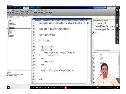
So, this is the function. So, I just changes this the radian from the pi and then I have this data. And here you see that I am using the ramp function, right, is it not. So, and then I generate this ramp function over here, ok.
