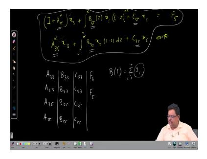
Similarly, if I do the same thing with respect to pitch, right, so then it should be I, because I indicate the that moment of inertia what this Iyy.  $(I + A_{55}^{\infty})\ddot{x}_5 + \int_0^{\infty} B_{55}(\tau)\dot{x}_5(t-\tau)d\tau + C_{55}x_5 = F.$
