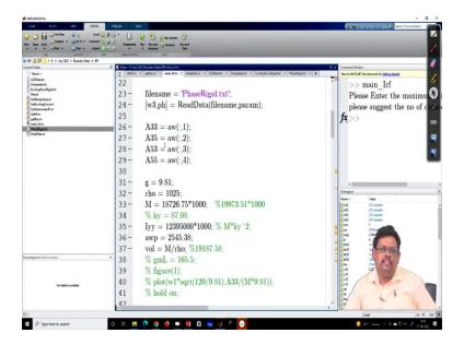
Now, here I just; so, initially is I am reading all this data that what is this damping data, the added mass data, the exciting force data, the phase, ok. And here I transferred into this *A33*, *A35*, *A53*, *A55*. Actually, you know if you solve this coupled equation of
