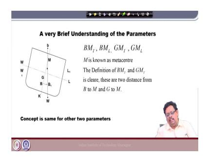
So, here similar thing actually, similar thing basically in case of a  $GM_L$  and  $BM_L$  also right? The concept is same that only thing is that instead of tilting in this location we tilting in this direction to find out that metacentre for that  $GM_L$  and  $BM_L$  ok.
