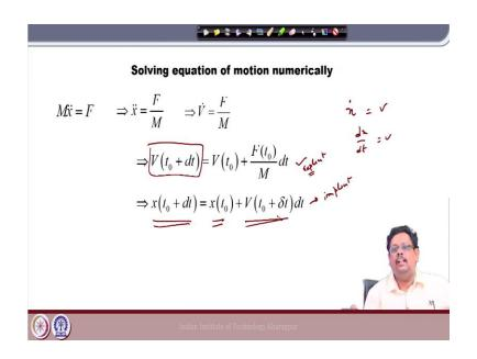
Now, here we are going to solve  $M\ddot{x} = F$ . So, now, I convert this into the first order equation which is  $\dot{V} = \frac{F}{M}$ . So,  $\ddot{x}$  is nothing but the  $\dot{V}$  right. Now I am using this Euler approximation scheme so, I can find out the velocity at the next time steps equal to velocity at the present time state plus the functional value.
