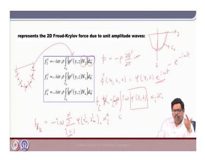
Now, here we are going to check that how we can get the sectional force. Now, in sectional force you know that it is force is nothing but the integration of the pressure. Now, where I going to do the integration now here this f since it is f is in the y z plane because, I am drawing the cross section.
