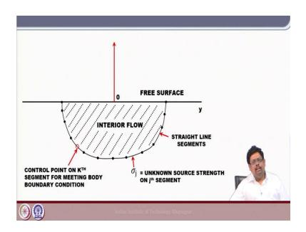
And now again it is the same it is a source panel method. So, initially this is the this is the strength is unknown and once you find out the strength and then you can from the this from this equation you can get the expression for the phi also right. So, again exactly the same right so, initially this we can call the strength and normally we define this as sigma. So, once we know this sigma and then we apply this sigma over here and then we know the value for the  $\phi$  right ok.
