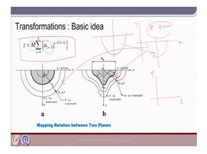
So, let us find out that what is the idea? Now, idea is that suppose I have a ship shape body which is here. So, let us say I have a ship shape body and now it is in basically my z plane. So, this is in z plane and I try to find out the added mass and damping of a ship shape body. So, so here I know that this there are some cross sections are like this and that you find out what is the added mass of this.
