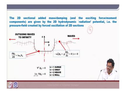
So, now, here I you know in a graphical way I said the same thing, now here you have in this body you must have this body boundary condition right and here in the free surface you have this free surface boundary condition right and then at the bottom definitely the bottom boundary condition right. So, this is the whole picture.
