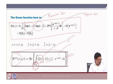
Now, third is the now this is the Green's function I called the free surface Green's function. Now, here you can see we have this log term right so; that means, that this is the Rankine part this is the called the Rankine part of the Green's function and this is called the regular part right.
