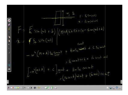
So, it is again a very simple thing that suppose you have a. So, what is the radiation force or is nothing but in calm water you are oscillating a body in some frequency right. And then some pressure field generated around this body if you integrate the pressure field you will get the radiation was fine.
