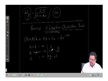
So, we write this  $\omega_z$  is nothing but the restoring coefficient C divided by mass plus added mass right. Now, you see like now suppose you have a you know frequency of encounter like or that frequency of the oscillation of the forcing function is  $\omega$  and this is of course, your, the natural frequency  $\omega_z$ .
