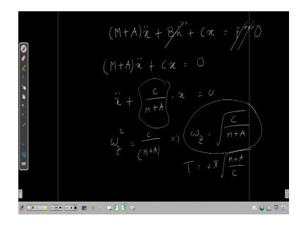
So, we write  $(M + A)\ddot{x} + B\dot{x} + Cx = F^{exe}$ . So, this is the fundamental equation right.
