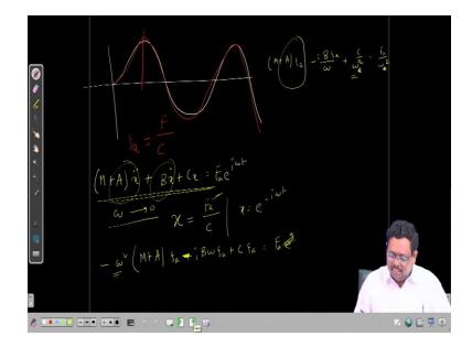
It means that when you are in top ok. And then this is exactly what is happening in the low frequency region right ok so; that means, there is no phase first of all and second you are moving with the wave. Now if you see that what is happening you see that that response  $\xi_a$ , is equals to that amplitude of the exciting force divided by the linear restoring component.
