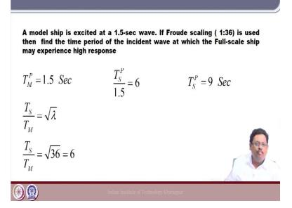
Now, it is written that a model ship is excited at 1.5 second wave. Now, if you maintain the Froude scaling 1:36, so that means, that that lambda scaling of lambda is 1:36 ok. So, then if it is used; that means, it means that that length of the ship by length of the model equal to 36, right that is what the meaning of 1 is to 36 scaling. So, the question is asked that what the time period of the incident wave at which the full scale ship maybe experience high response.
