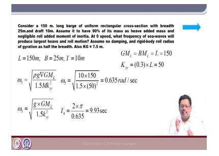
So, this is the given to you L = 150m, B = 25m, T = 10m. Now, what I approximate first that at and pitch added moment of inertia maybe the 50 percent of the you know that moment of inertia pitch moment of inertia. So, added moment of inertia I take is a 50 percent of this. So, therefore, in the denominator I am taking  $1.5Mk_{yy}^2$ , ok.
