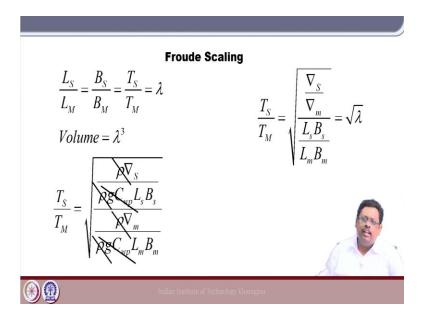
So, let us come back to our topic which is the Froude scaling. Now, when you do the experiment normally you are doing in the model scale. A ship normally conventional ship the length would be the scale of 150 - 200 meter long, right.
