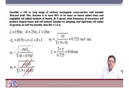
This, ok. So, it says that consider a 150 meter long barge I mean uniform rectangular cross-section. So, that means, that each cross sections it is uniform and it is 25 meter and then the draft is 10 meter and assume that we have a 90 percent of the mass can be considered as a added mass, right.
