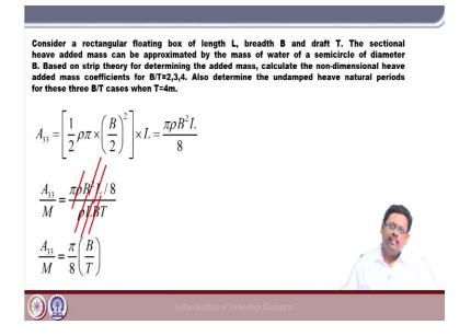
So, this is the problem we have the rectangular again we have rectangular barge with the length is L, B and T and it is given that the sectional added mass is given to you which is the which is the area of the semicircle whose diameter is equals to the beam, right. So, now, then you have to find out the added mass coefficient with respect to B/T ratio. So, this is the problem.
