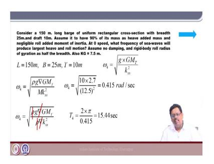
So, this is the basic parameters L = 150m, B = 25m, T = 10m and this is the formula for the natural frequency  $\omega_4 = \sqrt{\frac{\rho g \nabla G M_T}{Mk_{xx}^2}}$  in the roll.So, again I substitute M by the  $\rho \times \nabla$ ; that means, the volume or  $\rho$  into  $\nabla$  and then if I cancel the similar terms here also the  $\rho$  and  $\nabla$  will cancelled out. So, finally, I have this  $\omega \times g \times G M_T \times k_{xx}^2$ .
