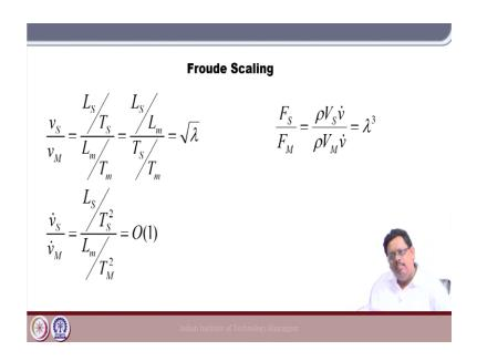
Now, we are doing the velocity. Now, velocity is the L/T, right. Now, I just rearrange it  $L/T = \frac{L_S}{L_M}$ ; that means, the ratio between the actual ship by model ship length divided by
